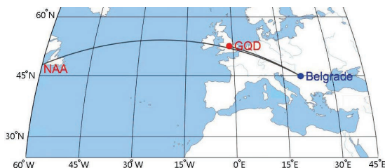
Figure 1. Map with analysed VLF signals' GCPs (black lines) emitted towards BEL receiver site (blue circle) from USA (NAA/24.0 kHz) and UK (GQD/22.1 kHz) (red circle).
