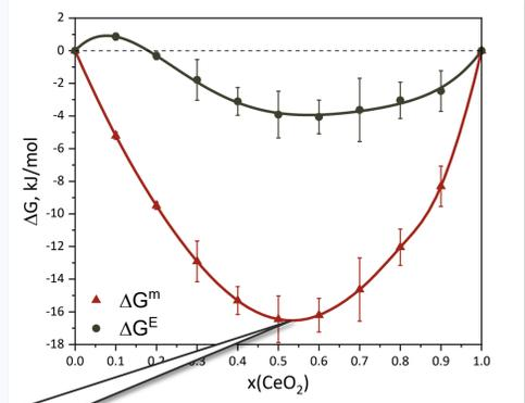
The dependence of ΔG<sup>m</sup> and ΔG<sup>E</sup> on ceria mole fraction at 2150 K
