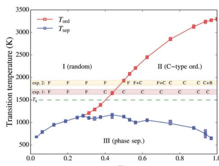
Theoretical phase diagram of the CeO<sub>2</sub>-Gd<sub>2</sub>O<sub>3</sub> system compared to experimental results<sup>4</sup>
