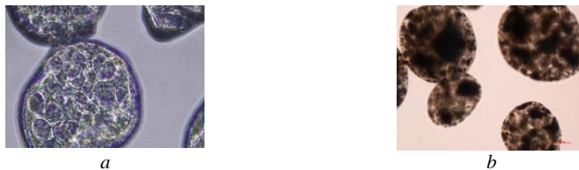
Figure 1. Light microscope view of microspherical cellulose nonmagnetic particles (a) and loaded by SPIONs (b), magnification x40.
