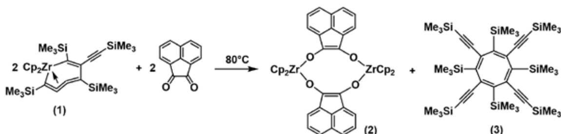
Figure 1. Reaction of complex 1 with acenaphthoquinone
