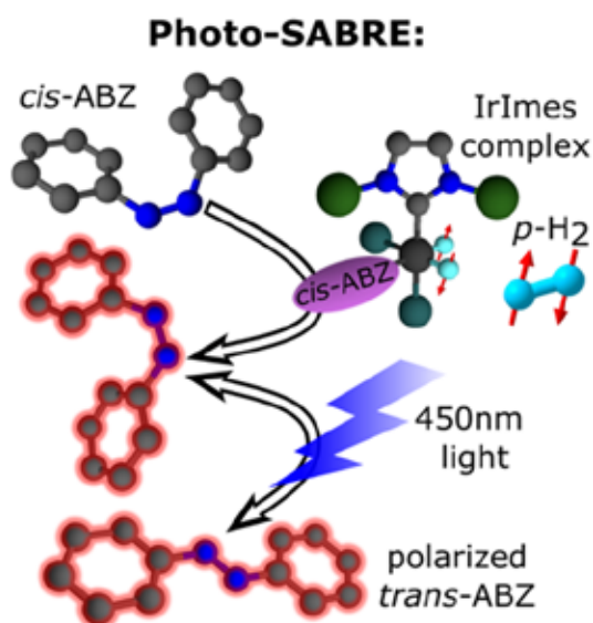
Figure 1. General scheme of polarization transfer to trans-azobenzene via Iridium-Imes catalyst 2
