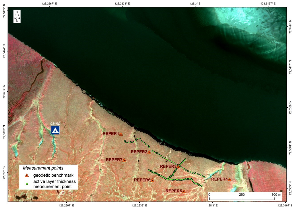
Figure 2.22.12: Location of active layer profiles and thaw subsidence benchmark measurements on Sobo-Sise Island (GeoEye-1 image on July 8 th , 2014, synthesis of NIR+Red+Green)
