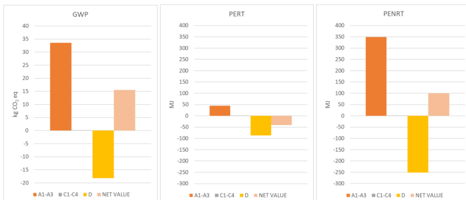
Figure 7. GWP (Global Warming Potential), PERT (Primary Energy Renewable Total) and PENRT (Primary Energy Non-Renewable Total) of aluminium alloy roofing systems related to the stages A1-A3, C1-C4, D. The net value is the sum of the impacts of all stages (source: ISCOM, 2022).
