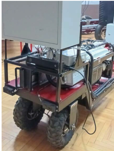
Fig. 2. Autonomous agricultural robot with installed depth sensor.
