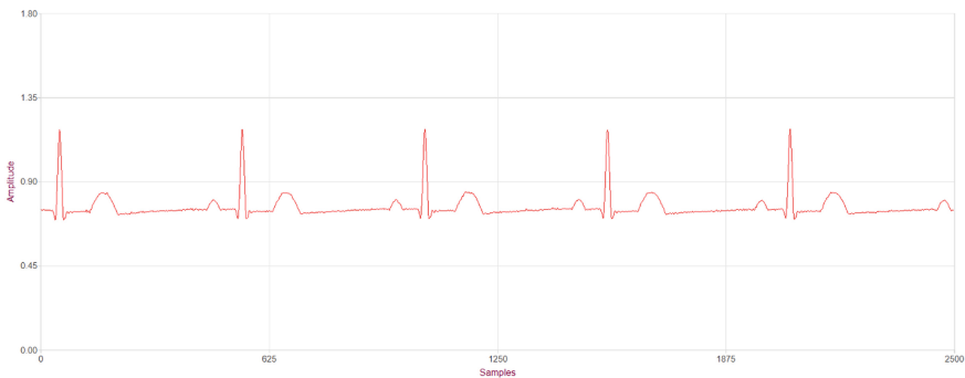
Fig. 10. FECCG test on an ECG signal generator
