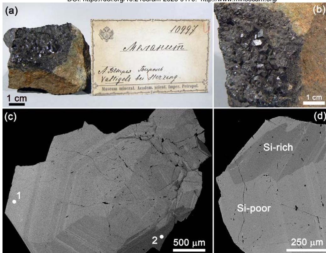
Figure 1. The studied tourmaline: (a) crystals (black) in bedrock (with label), (b) equant crystals, (c) dissolved Si-rich zones (dark) inside Si-poor crystal (BSE-image), (d) Si-rich zone inside Si-poor crystal (BSE-image). Number are as in Table 1 and Figure 2
