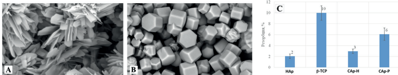
Fig. 1. A Plate-like carbonated apatite, CAp-P; B Hexagonal carbonated apatite, CAp-H; C Comparative efficiency of resorption in vivo for HAp, \beta -TCP, CAp-H, CAp-P
