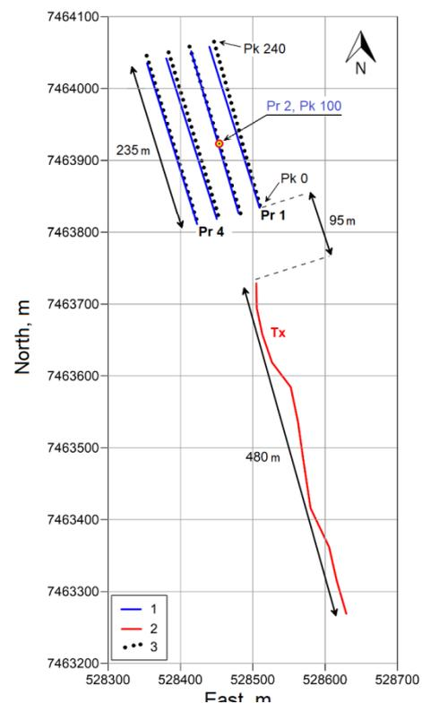
**Figure 1** Scheme of measurements. 1 – ERT profiles, 2 – CSRMT transmitter line, 3 – CSRMT stations. The yellow-red circle marks PK-100 on profile 2.
