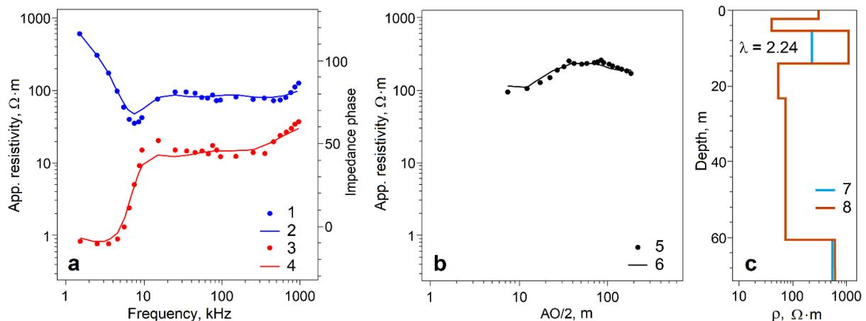
**Figure 2** Results of the joint 1D anisotropic inversion of ERT and CSRMT data for PK-100 in the profile 2. a) CSRMT curves: 1 -  $\rho_a$  field curve, 2 -  $\rho_a$  model curve, 3 - phase field curve, 4 - phase model curve; b) VES curves for the three-electrode AMN array: 5 -  $\rho_a$  field curve extracted from ERT data, 6 -  $\rho_a$  model curve; c) 1D anisotropic model: 7 -  $\rho_H$ , 8 -  $\rho_V$ .
