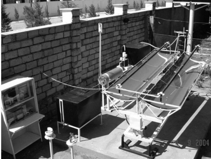
Fig. 4.1 General view parabolic trough solar energy concentrator
