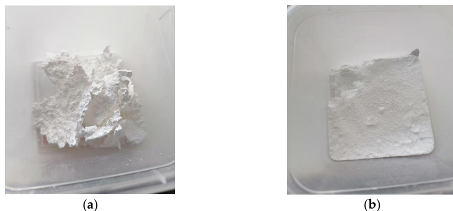
Figure 2. Samples obtained with different solution concentrations: (a) sample 2.1, concentration 32.6%; (b) sample 6.1, concentration 8%.
