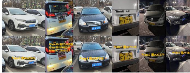
Figure 4. Visualized results. The first line displays the input original image, the second line displays the recognized license plate type and license plate number
