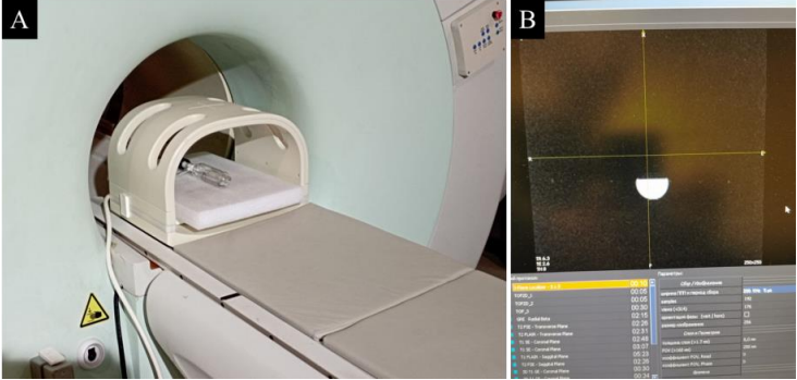
Figure 1. A: photo of the first phantom inside the receiver coil. B: ^{19}\text{F} MR image of the phantom in axial projection
