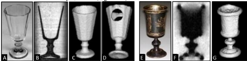
Figure 2. MRI of a glass goblet (B, C, D) and copper-silver goblet (F, G). A and E - photos of the goblets; B, F - central slices of the MR images; C, D, G - volumetric reconstructions 3D rendering
