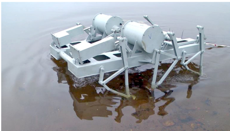
Fig. 1. Underwater walking vehicle (modular hardware complex) MAK-1
