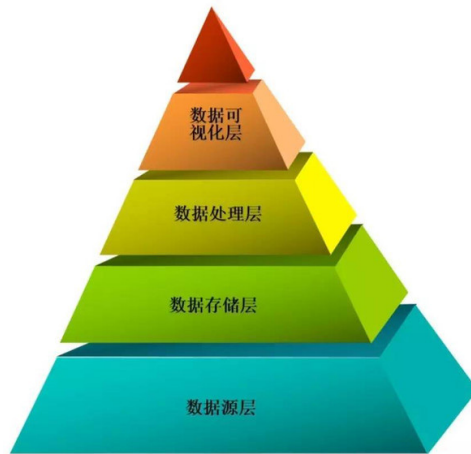
Fig. 2. Visualisation framework structure. There are 5 layers, from bottom to top: data source layer, data storage layer, data processing layer, data visualisation layer
