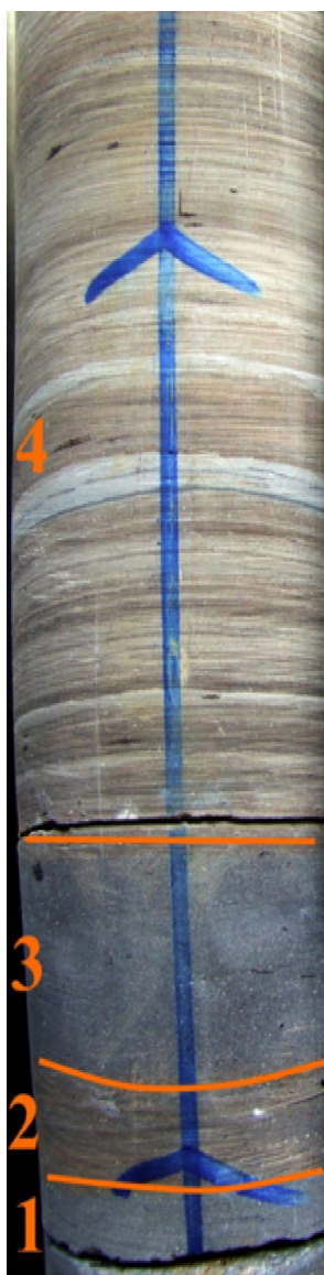
Fig. 1. Drilled core from the borehole at approximately 630m; 1 and 3 - sandy silts lack of pronounce lamination; 2 and 4 - brownish laminated fine-grained clastic rocks.
