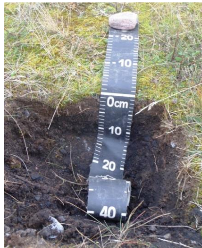
Figure 3. The photo of Petrozem (AY horizon) formed on rock material (Leptosol (Humic)—WRB).
