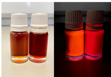
Figure 1 CdSe and CdSe/CdS CTs in daylight and in UV 365 nm.
